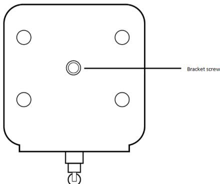
1. Bracket screw – this is the position to screw in the bracket of the EM6325. With the bracket, you can install the EM6325 on the wall.
