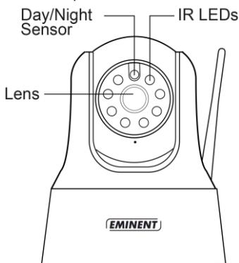
1. Lens – the lens is inside the camera body and the focus of the lens is fixed, you do not need to spend time to adjust the focus.
