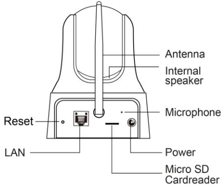
1. Power jack – this is the place to plug in the power adapter. The power needed for this EM6325 is 5V/2A, please make sure you are using the correct power adapter.
