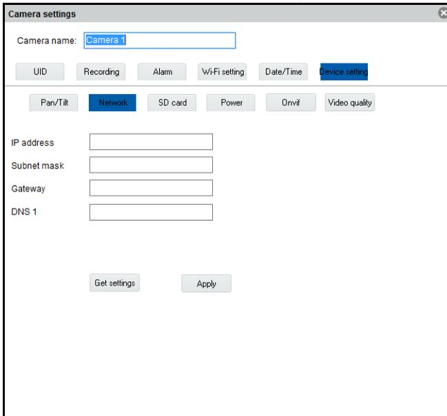
The screenshot shows the 'Camera settings' window with the 'Network' tab selected. The 'Camera name' field contains 'Camera 1'. The navigation tabs include UID, Recording, Alarm, Wi-Fi setting, Date/Time, Device setting, Pan/Tilt, Network (selected), SD card, Power, Onvif, and Video quality. The Network settings include: 'IP address', 'Subnet mask', 'Gateway', and 'DNS 1', each with an empty text input field. 'Get settings' and 'Apply' buttons are at the bottom.
