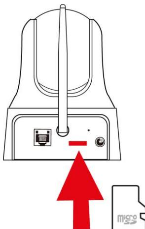
*Note: When you plug in the micro SD-card while the camera is powered, please reboot the camera for the micro SD-card to work properly.*
