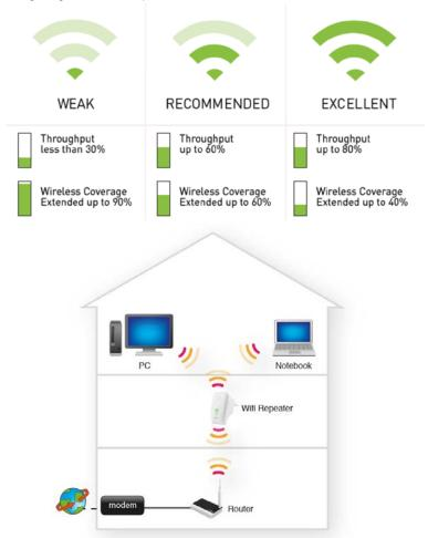
Hint: Before placing the EM4595 on its destined location, the device needs to be setup. Setting up the EM4595 wireless repeater can be done best, if the EM4595 is located near your wireless router. After setting up the EM4595, you can place the EM4595 at a location defined by using the signal indicator LEDs and the recommended setup as described previously.
