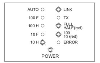
3. The tested device is a 100 BASE-TX full-duplex device capable linked at 100Mbps in full-duplex mode. It is also transmitting an auto-negotiation packet.
