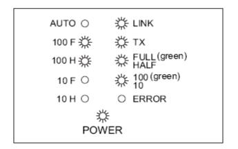
4. The tested device is a 10 BASE-T, half-duplex device, linked at 10Mbpsin half-duplex mode and is communicating bad packets.
