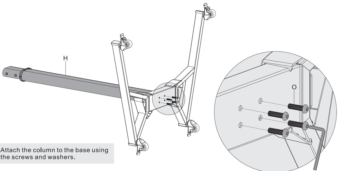
Attach the column to the base using the screws and washers.
