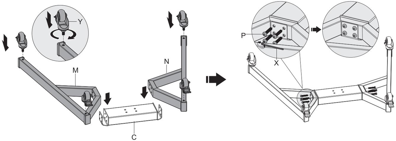
Attach the right base to the middle base and secure with screws(P). Repeat this step for the left base.
