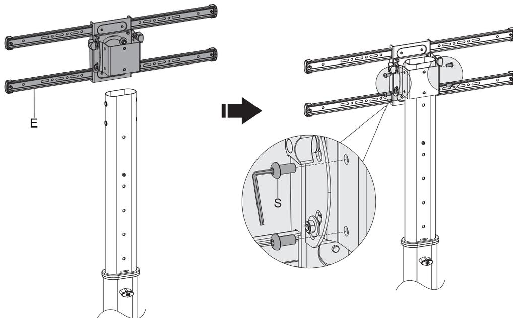
Attach the universal plate to the column using the appropriate screws.
