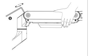
Before adjusting the spring tension and during the adjustment process, position and hold the arm horizontally as shown. Use the supplied Allen Key for adjustment. Ask for assistance should you reauire it.
