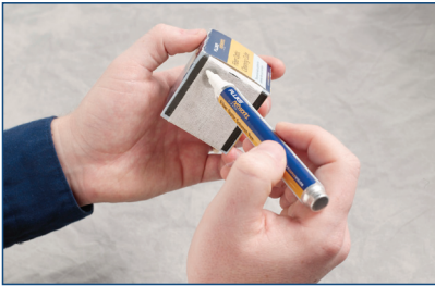
Holding the connector perpendicularly, swipe the end-face from the wet spot into a dry zone.
