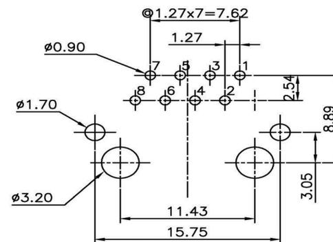
PC Board Layout  $t=1.6\text{mm}$
