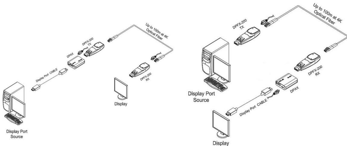
DPAX can improve transmission length of DPFX-200 via optical fiber. It has been confirmed that DisplayPort signal transmission length has improved up to 300m when using DPFX-200 with DPAX under certain environment such as below configuration. Each 200m and 300m of DisplayPort signal transmission has successfully tested when using GTX960 as a display source and ASUS PA328Q as a display.
