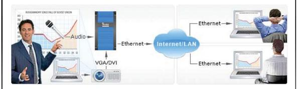
The VGA Broadcaster Lite is able to broadcast video in resolutions at up to 1600 x 1200 without any loss in quality or sharpness. The broadcasted video stream is then viewed with a media player such as QuickTime or VLC.
