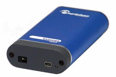
Being a single-purpose frame grabber, the DVI2USB Solo is fine tuned for the capture of digital single link DVI signals only. This means that the DVI2USB Solo can grab images from any DVI source with a resolution of up to 1920x1200. What's more, the performance-oriented DVI2USB Solo is able to achieve capture rates at up to 30 frames per second without any loss in picture quality.
