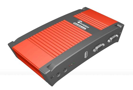
VGA2Ethernet PRO is a compact external VGA frame grabber that is capable of capturing VGA signals at rates of up to 120 frames per second. Designed for high speed and high precision military, medical and industrial applications, Epiphan Systems VGA2Ethernet PRO uses the common RJ45 Ethernet port to interface itself with the target computer, allowing for up to 1 Gigabit transfer rates.
