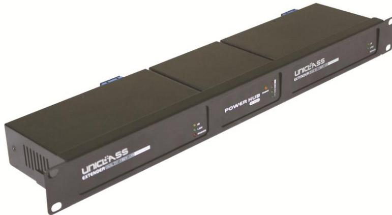
With optional mounting chassis and power hub (See above image), two transmitters can be mounted on the server rack for central management. The power hub provides two transmitter power connections using special power cable (Optional. See below cable image.) This optional mounting set provides a neater and more convenient way for mounting and managing transmitters on server rack.
